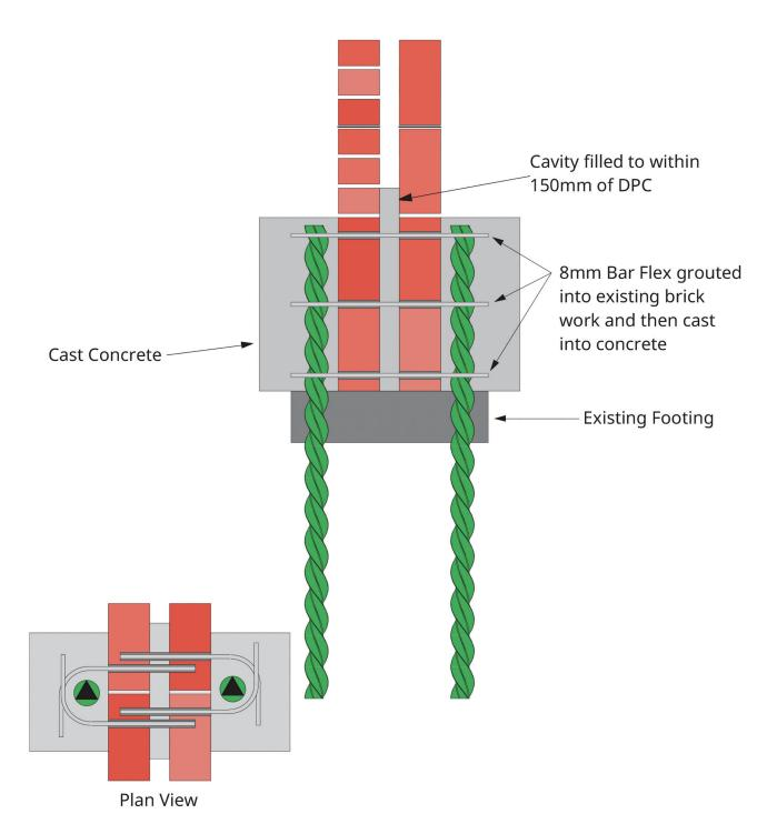
Showing way of fixing the reinforcement
