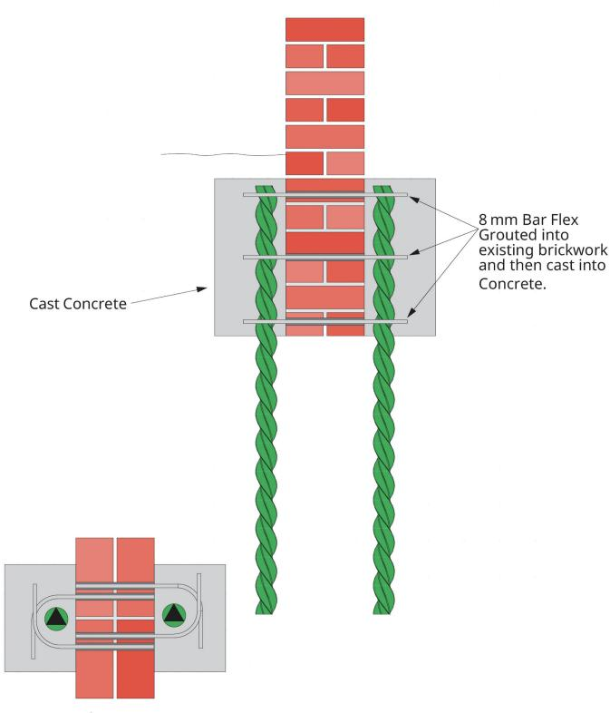
Plan View Showing way of fixing the reinforcement
